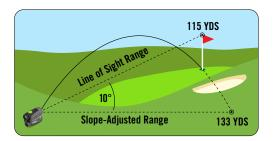
**Note:** When Slope Mode is off, the external green LED indicators will be off and the laser rangefinder is tournament legal.
